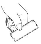
To protect electronic parts, discharge static electricity from your body by touching a water pipe (faucet) or other large metal object before handling the memory module. Or, wear an antistatic wrist strap, if possible, when you install the memory module.
